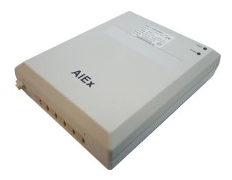
The AlEx (Alarm Extender) device is a telecontrol system that transmits local alarm signals via its G.703 64kbit/s interface to a remote alarm controller unit, which outputs the alarm via relay contacts. It enables to manage and supervise alarm systems, fire detection systems or similar devices via parallel I/O ports.
