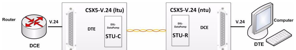
Figure 4-9 DTE--DCE Configuration
