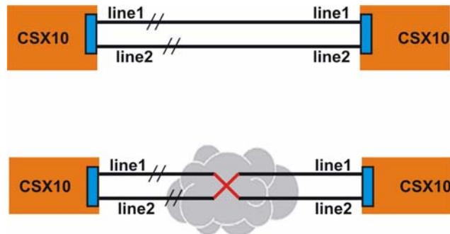
**Figure 4-4** Cross-Over of Copper Lines in n-wire mode
