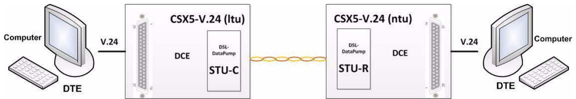
Figure 4-8 DCE--DCE Configuration (Default)
