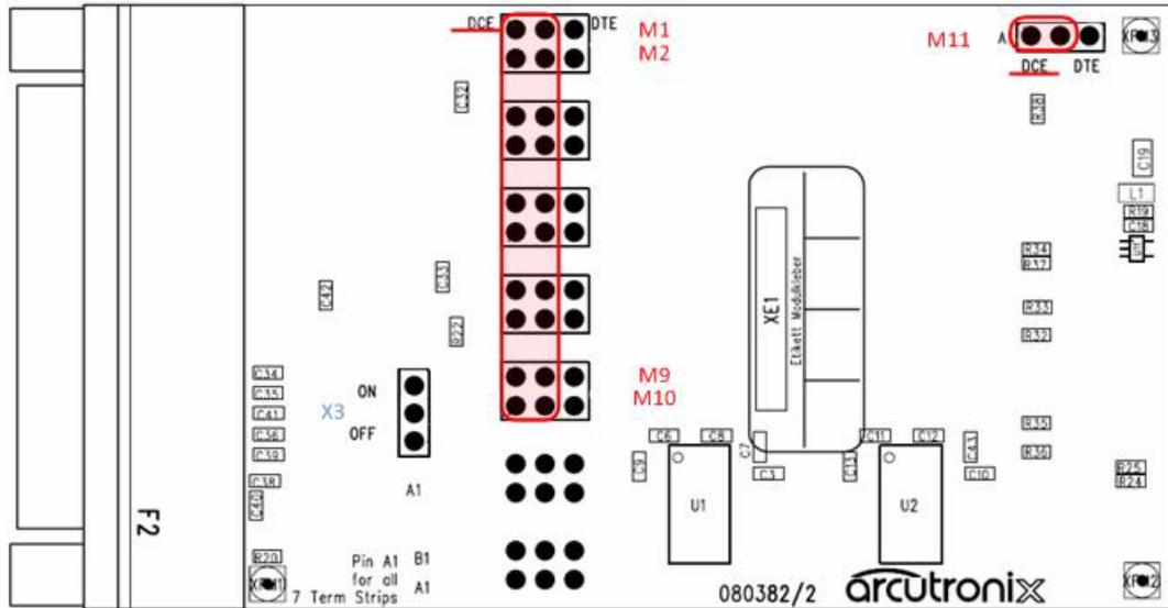
Figure 3-2 V.24 Interface Board, DCE Configuration
