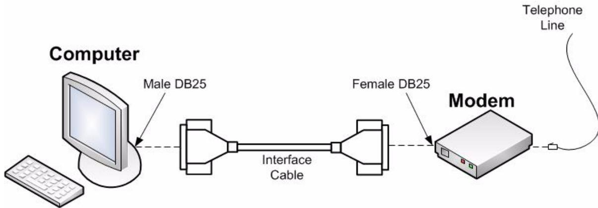
Figure 4-7 DCE and DTE
