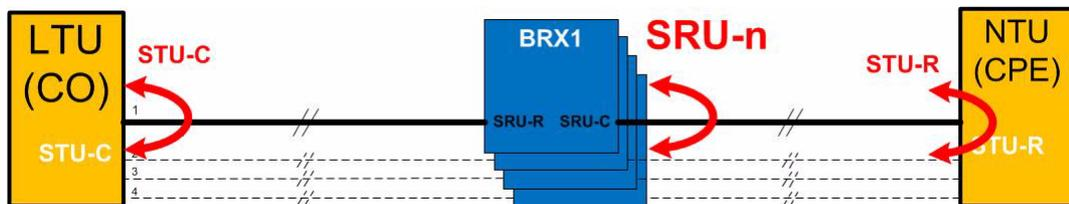
Figure 4-6 SHDSL Loops for CSX with Repeater
