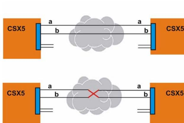
**Figure 4-3** Cross-Over of Copper Pair within one Line
