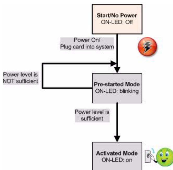
**Figure 4-12** Flow Diagram Power Management
