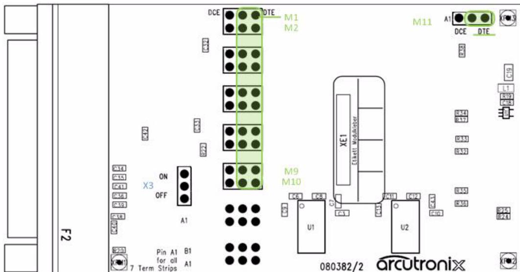
Figure 3-3 V.24 Interface Board, DTE Configuration
