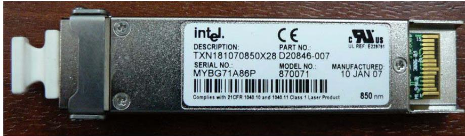
Figure 3-4 XFP Transceiver
