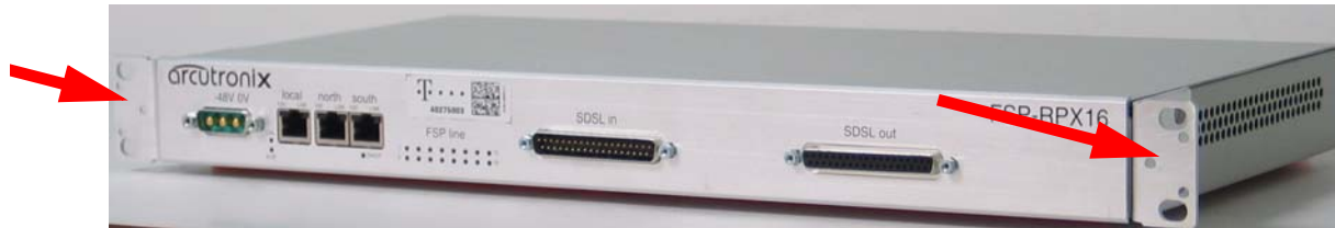
Figure 2-1 Rack Mount-Angles 19-Inch
