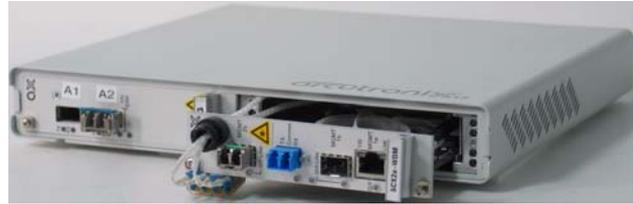
4. Fix the SCX2e to the housing using the provided screws.
