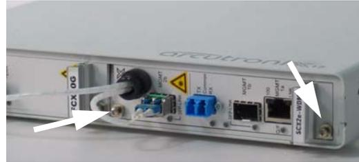
5. Connect the interface cables to the SCX2e.
