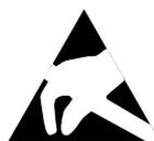
**CAUTION:** Discharge of static electricity (ESD) can damage or degrade electronic components. The electrostatic potential of a person can be several thousand Volt and a discharge to semiconductor components may have severe consequences. Observe the precautions below when you are handling any hardware with electronic components.
