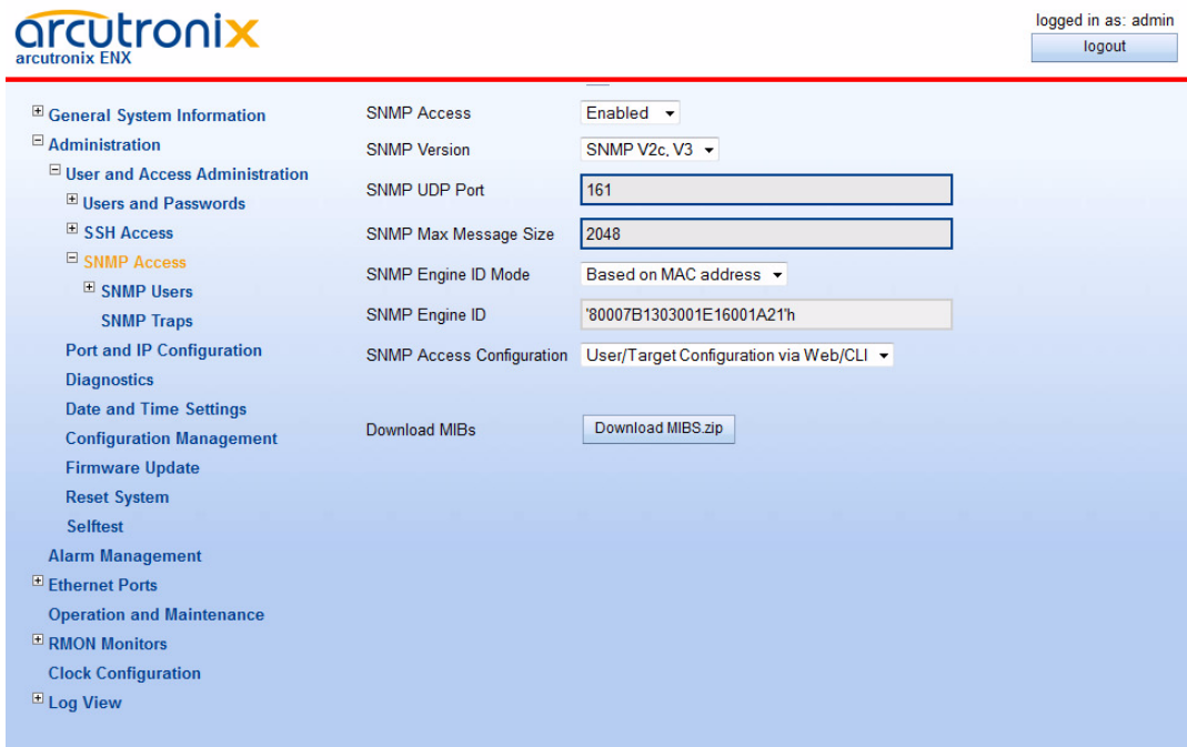
Figure 1-15 SNMP Configuration, SNMP enabled
